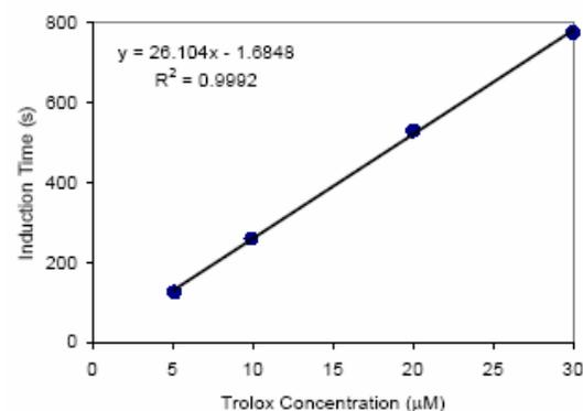
Figure 1: Time courses of luminescence in the presence of different concentrations of Trolox. A standard curve is obtained by plotting induction times vs. trolox concentrations in the final reaction mixture.
